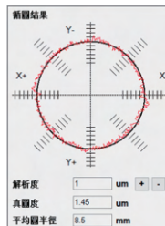
Reversal spike with compensation 1.5 μm
